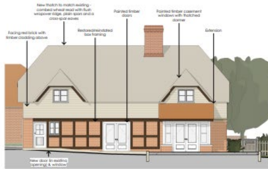
House 2 (Crocketts) - West Elevation as Proposed 1 : 100
