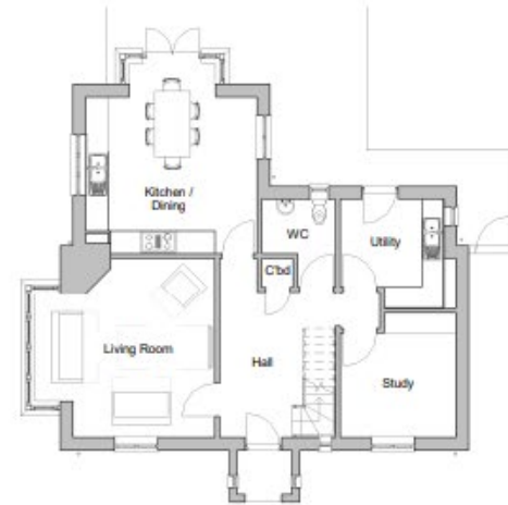
House 3 - Ground Floor Plan as Proposed 1 : 100
