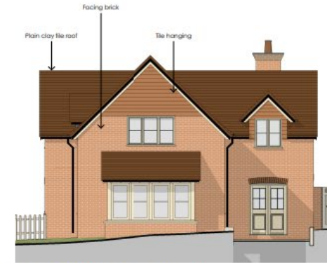
House 4 - South Elevation as Proposed 1 : 100
