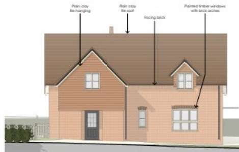
House 1 - West Elevation 1:100
